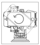
Adjust cradle in any angle with ball pivot joint.
