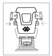
Press the Side buttons into locking position.
